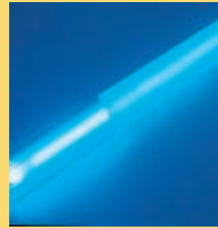
photo shows UV light blocked by fouling on one half of the quartz sleeve (A typical problem)
